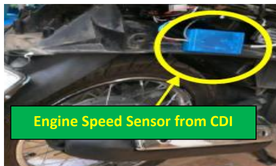
Figure 2.12 Engine Revolution Sensor from Capacitor Discharge Ignition
