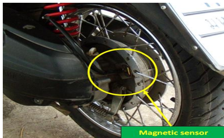
Figure 2.9 Magnetic Sensor on Rear Wheel of Motorcycle
